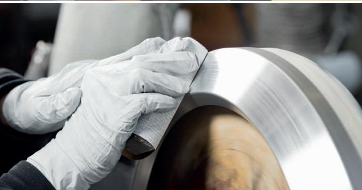
The CONVERSIO lamp shade is fabricated from a compressed piece of aluminium. During this process, a circle-shaped piece of sheet metal is rotated and pressed against a negative mold to give it its seamless volume.
